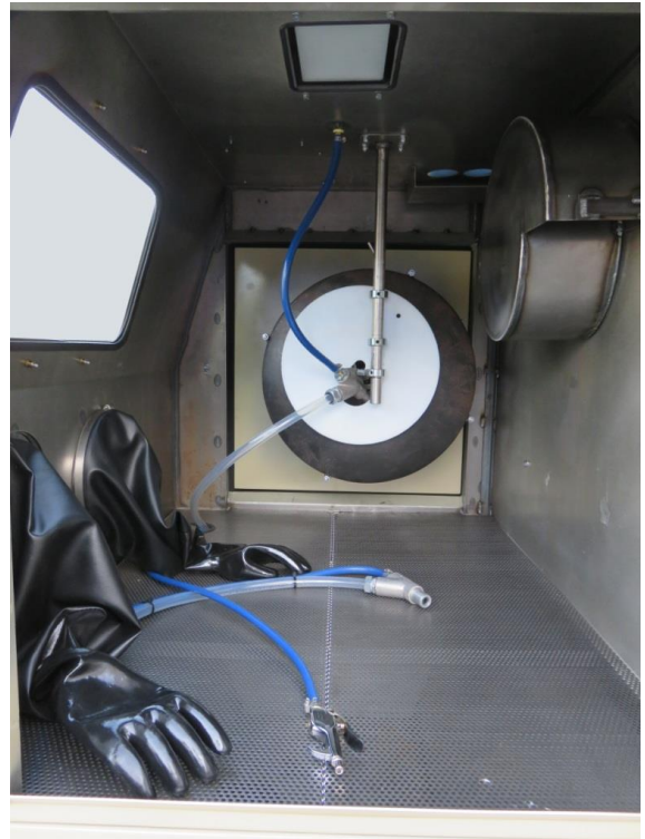
N-200 showing TB-2 with offset manual blasting station and optional pop out shield.
